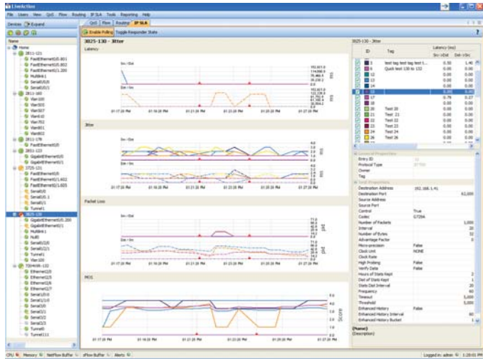
LiveAction IP SLA chart showing graphical view of real-time test data (center) and test properties in tabular format (lower right).
